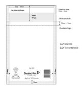
Dimension inside Dimension outside Tolerance 180 x 260mm 200 x 270mm +/-6mm
